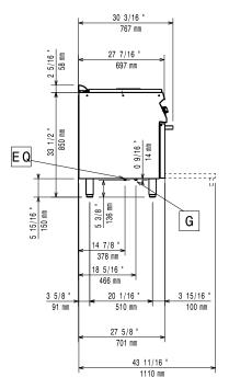
EQ = Equipotential screwG = Gas connection
